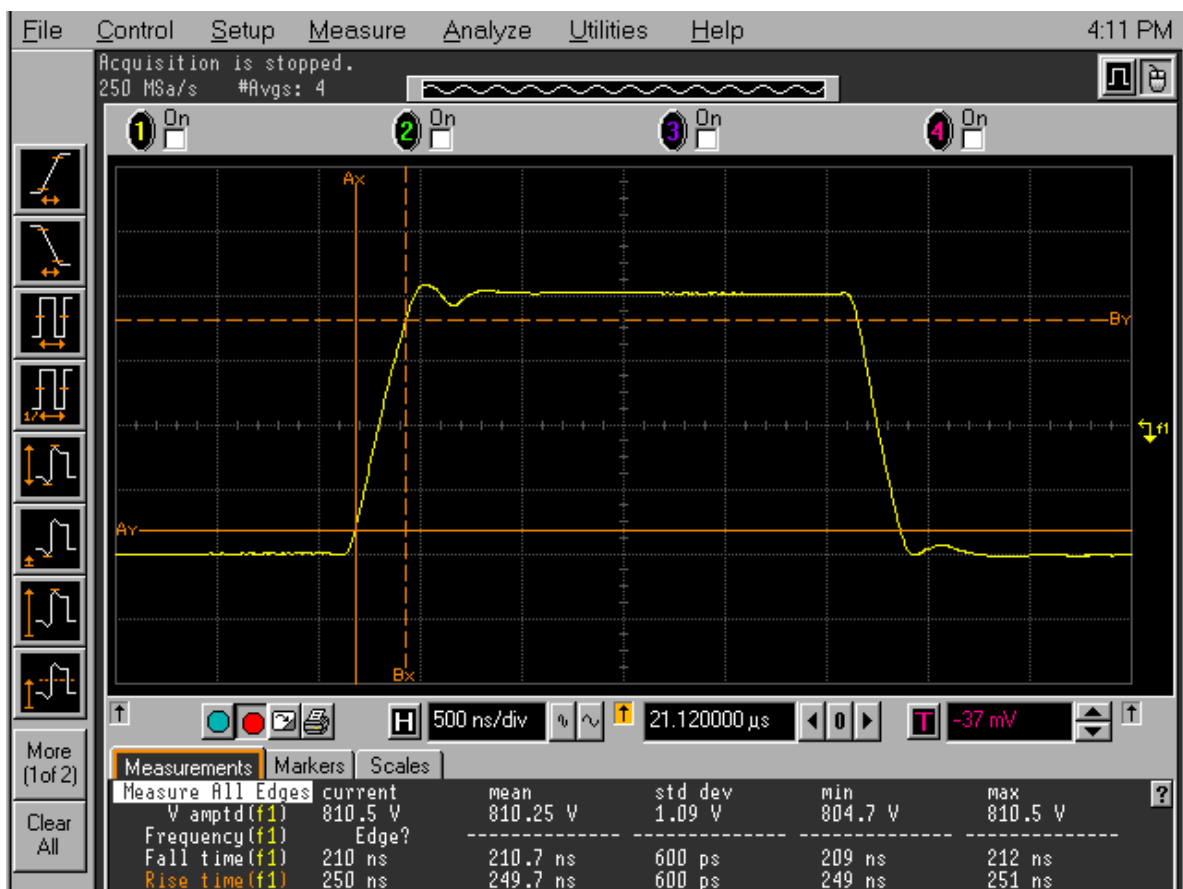
Typical rise and fall times at 1000V output
